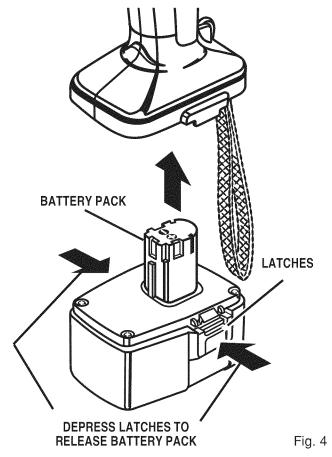
Make sure the latches on each side of your battery pack snap in place and battery pack is secured in drill before beginning operation.
